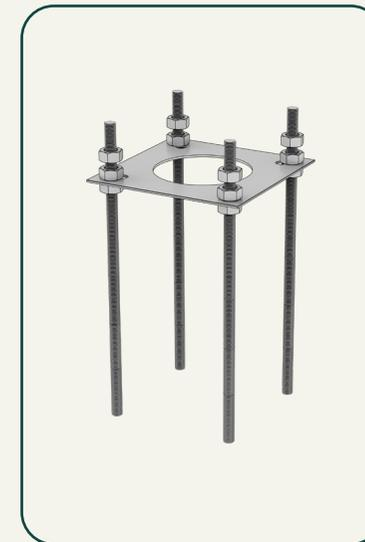
2. Place the hex nuts as shown in the image above. The top hex nut serves as the adjustment nut for leveling the pedestal, while the bottom two nuts act as locking nuts for the anchor plate
