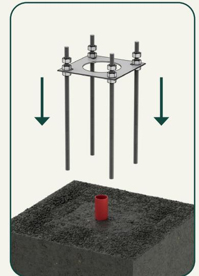
3. Place the anchor frame and cable conduit into the wet concrete. Route the cable conduit through the center hole of the anchor plate, keeping it at least **50mm** above the base of the concrete
