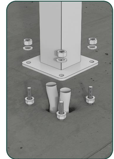
3. An alternative fastening method is to cast an anchoring frame in concrete. This also provides a stable and secure attachment for the pedestal. Please refer to the dedicated installation guide for this method
