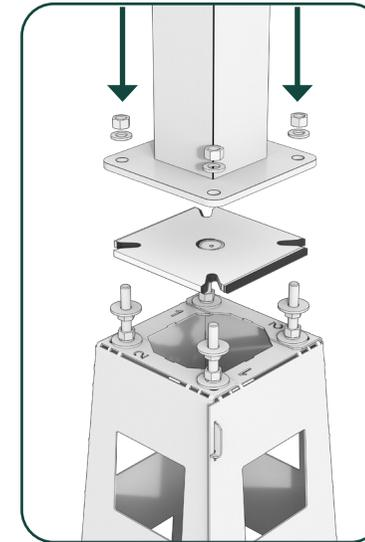
2. We recommend using a foundation (sold separately) for secure, robust, and well-drained anchoring of the pedestal.
