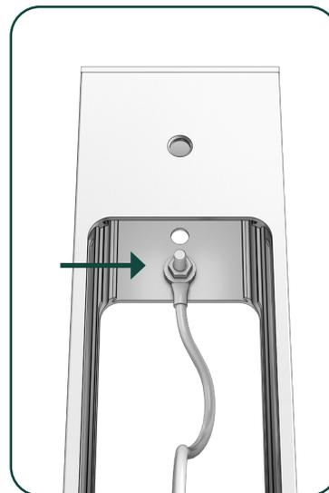
4. Perform the necessary wiring to the charging station(s) and ensure that the grounding of the pole is connected in the designated area
